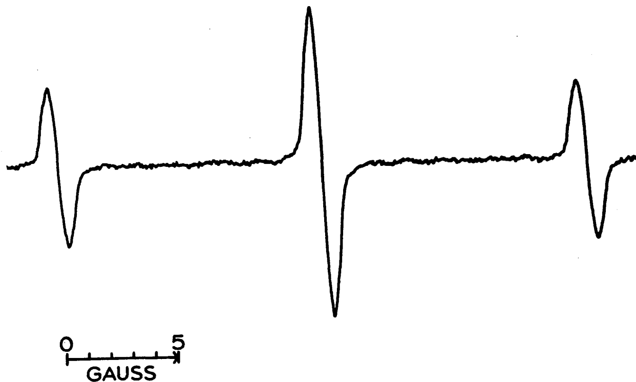
Figure 52. First derivative ESR spectrum of tricyclo[4.2.2.0 2,5 ]decane-3,4-semidione (LXIII) prepared by the in situ acyloin condensation of 0.2 M dimethyl cis -bicyclo[2.2.2]octane-2,3-dicarboxylate with sodium-potassium alloy in DME.
