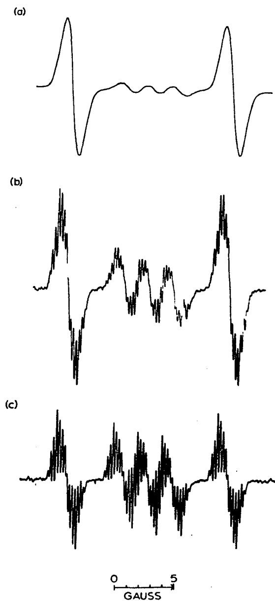
Figure 76. First derivative ESR spectra of the mixture of cis -1-methylbicyclo[4.2.0]oct-3-ene-7,8-semidione and cis -1-methyl-6-deuteriobicyclo[4.2.0]oct-3-ene-7,8-semidione prepared by the reaction of cis -1-methyl-7,8-bis(trimethylsiloxy)bicyclo[4.2.0]octa-3,7-diene (0.1 M) with potassium t -butoxide (0.2 M) in d_6 -DMSO; (a) spectrum recorded after 3 minutes; (b) spectrum recorded after 4 hours; (c) spectrum recorded after 7.5 hours.
